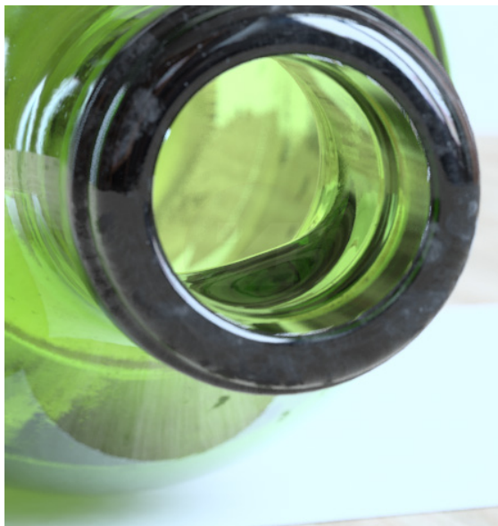
Slug in Neck- major defect.
